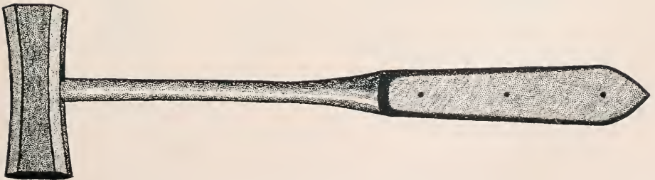
FIG. 35.—Steel hammer with proper handle. (One-half natural size.)
